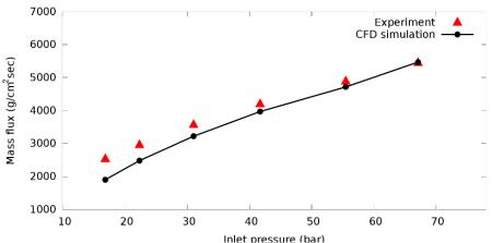
Subcooled nitrogen through a sharp-edged orifice (NASA TM X-71760)
