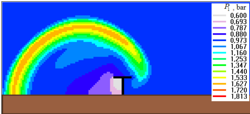
Figure 11. Pressure distribution in vertical section (case 4) at 0.0107 s
