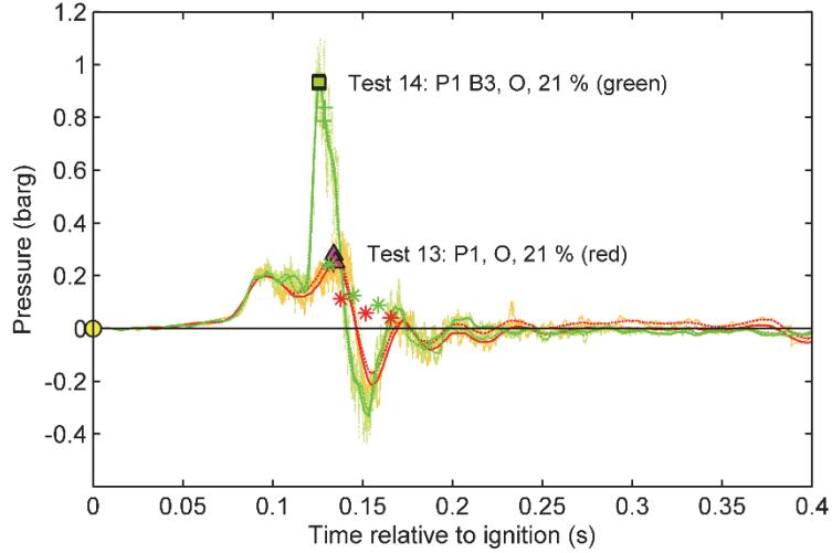
Figure 10. Pressure-time histories (P01 & P02) for tests 13 and 14.
