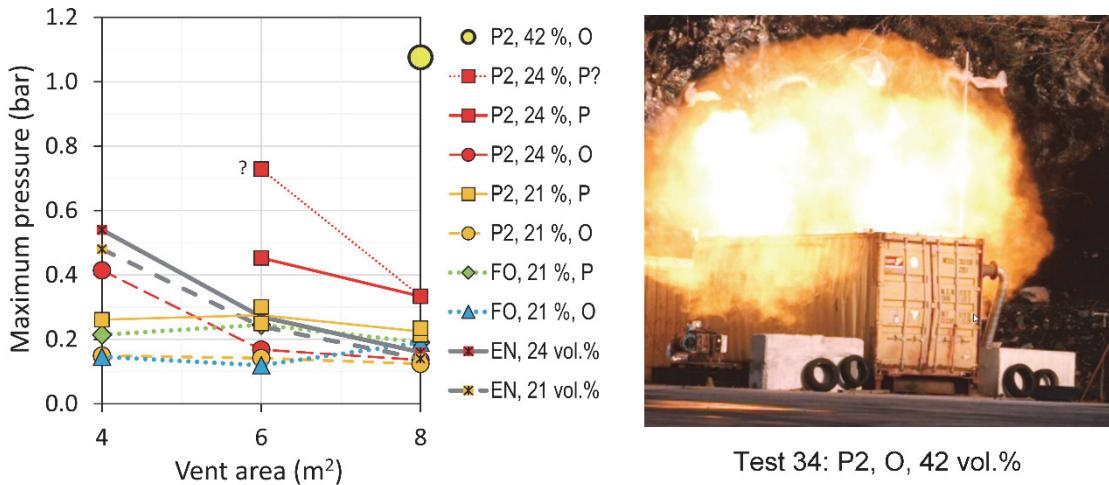
Figure 12. Maximum pressure vs. vent area for tests 15-34 (left) and vented explosion (right).
