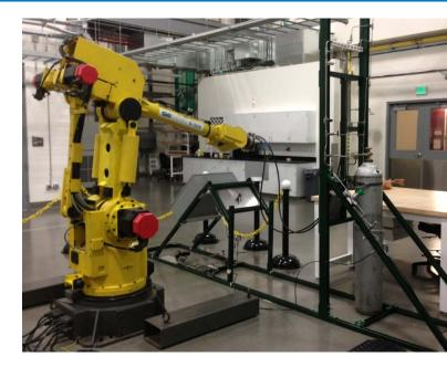
Long-duration accelerated life testing in hydrogen is accomplished autonomously to simultaneously stress the hose assembly with realistic fueling protocols (pressure, time, temperature) and the mechanical stress applied to hose during the process of connecting and disconnecting the hose to the vehicle during the fueling event.
