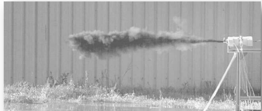
Powder expulsion cloud without external source of ignition
